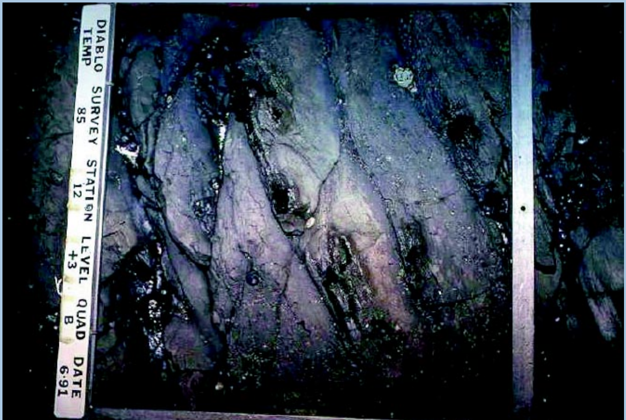
AFTER: The same quadrant photographed in 1991 after 5 years of thermal discharge from Diablo Canyon Nuclear Power Station showing bare rock, the complete reduction of a marine community throughout Diablo Cove.
